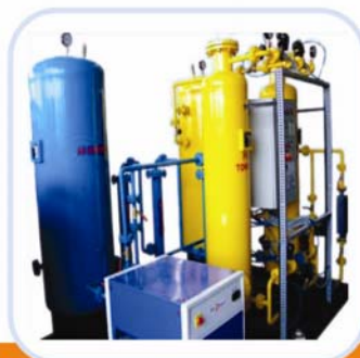
PSA Nitrogen Plant
